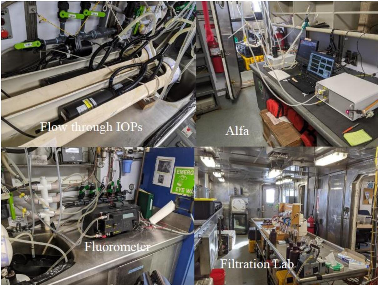
Figure 3. Instrument setup in the labs. Top left: flow-through system for IOPs; top right: ALFA system; bottom left: Fluorometer; bottom right: filtration lab.
