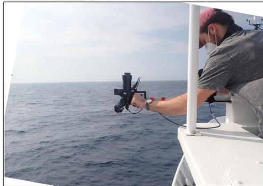
Figure 27. The Gybe optical sensor mounted to the port side of the R/V *Gordon Gunter*. Clemente Borgogni is measuring the water-leaving radiance with a field spectrometer at a cruise station. The Gybe instrument is in the center of the image and has two sensor heads. The vertical black tube contains the sensor measuring the downwelling irradiance, while the black tube facing the ocean measures the upwelling surface radiance.
