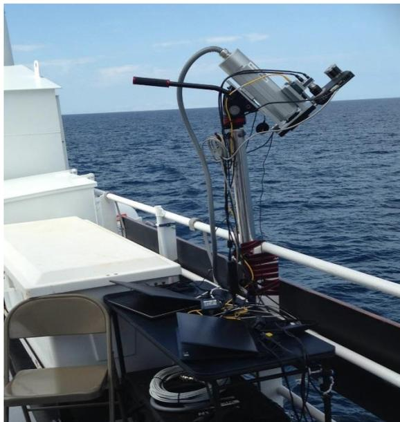
Figure 8. Snapshot hyperspectral imager with polarization camera on the ship.
