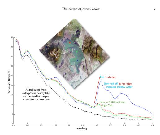
Fig. 6.  $\rm HICO^{TM}$  image for Klamath Lake, Oregon, 31 July 2011. The color of the spectra indicates where the sample location. A 'red edge' is seen in shallow waters. High chlorophyll levels are also indicated by the fluorescence peak. The dip near 430 nm in all the spectra is due to the G Fraunhofer lines in the solar irradiance.
