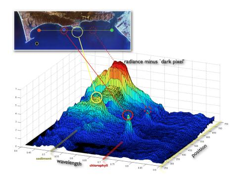
Fig. 7. HICO<sup>TM</sup> spectral surface for (yellow) line of spectra indicated in RGB image at top (Pt. Reyes), 28 September 2011. The 'dark pixel' (lower left) is subtracted from every spectrum, resulting in a spectra that better highlights extrema like those indicating Chlorophyll ( $\approx$ 700 nm) or sediment ( $\approx$ 500 – 620 nm).
