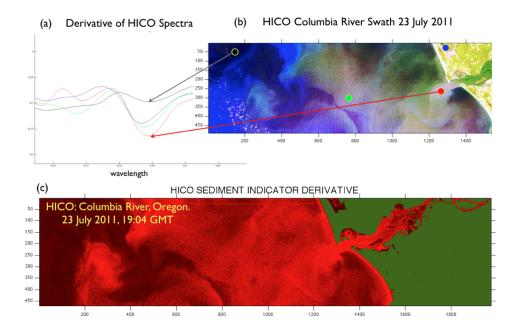
Fig. 9. Analysis of a HICO spectra using derivative spectroscopy. (a) The derivative spectra calculated at points indicated from a HICO image of the Columbia River (b) taken 23 July 2011. (c) A 'regionally tuned' map of sediment concentration (bright red is high sediment) emanating from the Columbia River.
