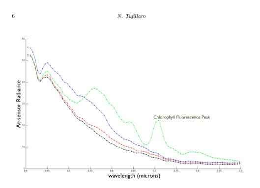
Fig. 5. HICO<sup>TM</sup> spectra for image of San Francisco Bay from 28 September 2011. The color of the spectra indicates where the sample location shown in Figure 4. The green spectra is from the salt ponds in the southern bay and show very high chlorophyll levels as indicated by the prominent chlorophyll fluorescence near 710 nm. The black spectra are from a relatively clear ocean point and shown a spectra dominated by Rayleigh atmospheric scattering.
