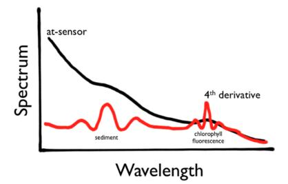
Fig. 8. Sketch showing how derivative spectroscopy can amplify narrow-band features in a spectrum. The  $4^{th}$  derivative of the spectrum is marked by red.
