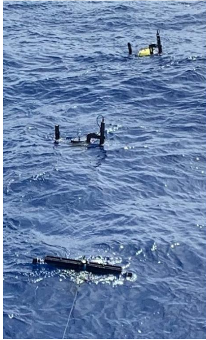
Figure 28. HyperNAV (front) in the surface buoy mode, with two HyperPro-IIs in the SBA configuration behind.
