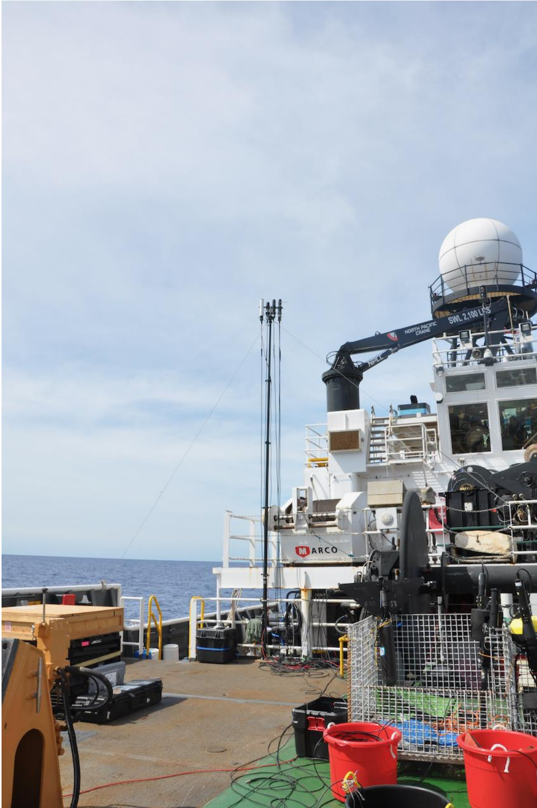
Figure 7. Above-water irradiance sensors mounted atop the telescoping pole.
