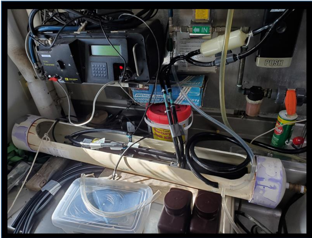
Figure 11. The NRL IOP continuous flow-through wet lab setup on the NOAA Ship Oscar Elton Sette included a hyperspectral ac-s instrument (non-filtered) and a BB3 sensor. The ac-s instrument was placed inside a PVC tube water bath to maintain a constant temperature during operation and was calibrated with Nanopure water before and after the cruise. The BB3 instrument was placed inside a flow cell. The PVC tubes and the BB3 flow cells were designed specifically for those instruments.
