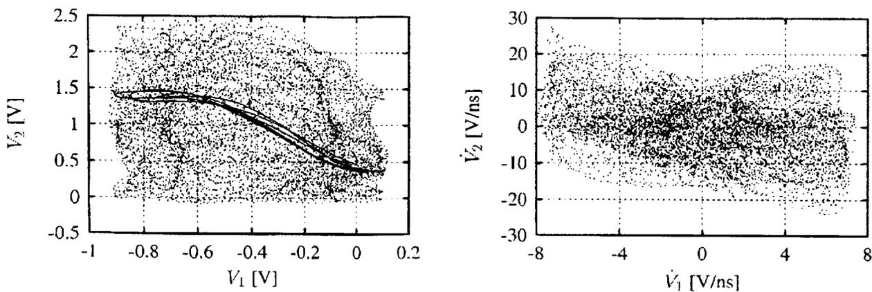
Figure 2: (left) Automatically controlled coverage of the  $(V_1, V_2)$  plane of a HEMT by 27 vectorial large-signal measurements. The solid line represents the case with no  $a_2$  present. (right) Corresponding coverage of the  $(\dot{V}_1, \dot{V}_2)$  plane.
