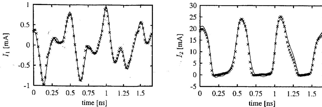
Figure 3: Comparison of the measured (x) and modelled (—)  $I_1(t)$  (left) and  $I_2(t)$  (right) of a HEMT under two-tone excitation.
