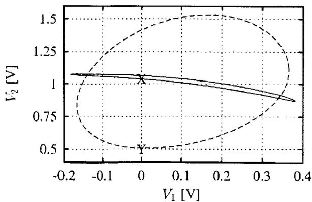
Figure 1:  $(V_1, V_2)$  voltage plane of a HEMT with the  $V_1(t) - V_2(t)$  characteristic if no  $a_2$  applied (solid line) and with the adequate  $a_2$  applied to cross the  $(0 \text{ V}, 0.5 \text{ V})$  point (dashed line).
