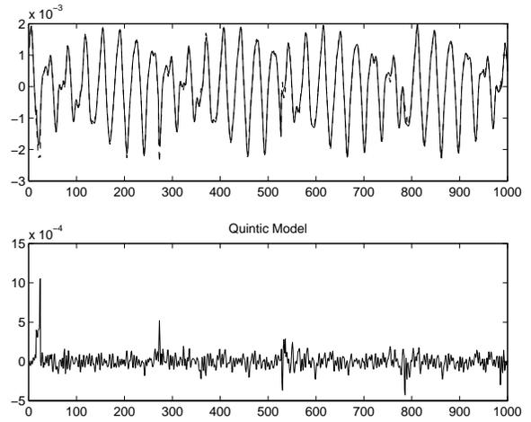
FIG. 9. The fit and errors of a quintic model for current 1.
